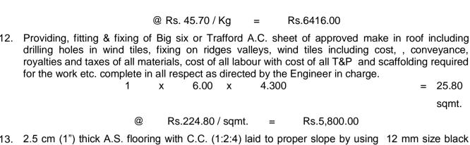
13. 2.5 cm (1") thick A.S. flooring with C.C. (1:2:4) laid to proper slope by using 12 mm size black hard crusher broken grantie stone chips of approved quality and from approved quarry including punning, watering and curing for 28 days with cost, conveyance, royalties and taxes of all materials, cost of all labour with cost of all T&P and scaffolding required for the work etc. complete in all respect as directed by the Engineer in charge.
